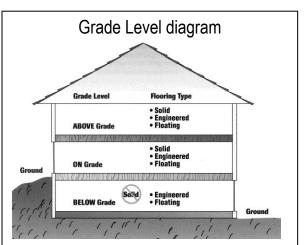
If the soil surrounding a structure is 3 inches or more above the floor of any level, consider that level below grade. This includes walk-out basements. In addition, the surrounding soil should be sloped away from the structure.
